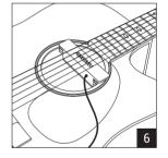
6. Connect the 1/8" jack on the cable to the pickup.
