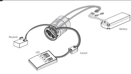
Use LED program box to set ESC parameters It is easy and fast to read and set parameters via a LED program box
