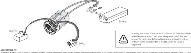
Insert the throttle cable of the ESC into the throttle channel of receiver. Because the red line of throttle cable output 6V/7.4V voltage to receiver and steering servo, do not supply power to receiver, otherwise the ESC may be naged. If need to supply power, pick out the red line among throttle cable, wrap it and suspend. Connect battery
