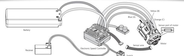
This is an extremely powerful brushless motor system. For your safety and the safety of those around you, we strongly recommend removing the pinion gear attached to the motor before performing calibration and programming functions with this system. It is also advisable to keep the wheels in the air when you turn on the ESC.
