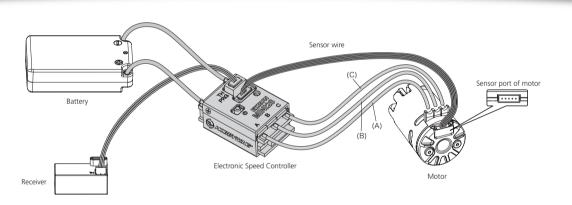
This is an extremely powerful brushless motor system. For your safety and the safety of those around you, we strongly recommend removing the pinior gear attached to the motor before performing calibration and programming functions with this system. It is also advisable to keep the wheels in the air when you turn on the ESC.
