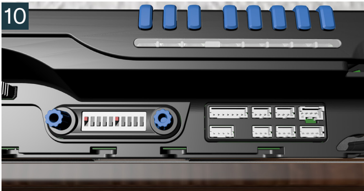
10 Plug the AutoSwing into a 110V outlet. Before powering the operator ON, set DIP Switch #1 to OFF and DIP Switch #6 to the ON positions.
