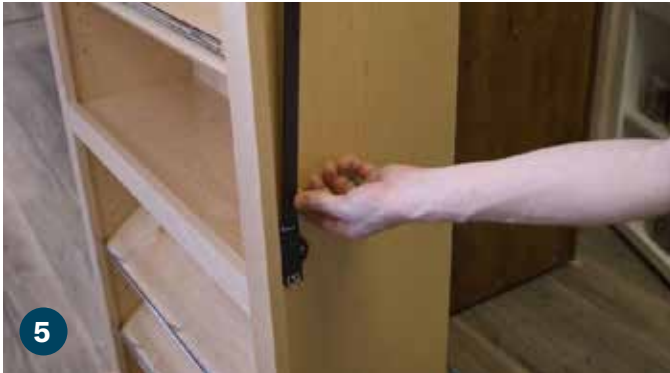
Slide (3) lock bar brackets onto the top lock bar and place the bar in the lock.
