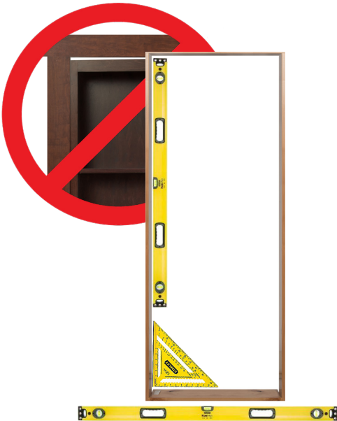
Move lower jamb out half pop distance.
