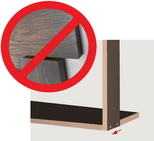
Move lower jamb out half pop distance.
