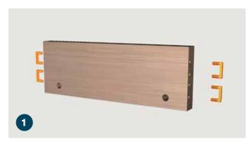
Insert (4) dowel pins (A) all the way into the back top, back middle, and back bottom. Some splitting may occur but will not effect the performance or appearance of the door.
