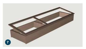
Dry fit the face frame onto the bookcase to ensure that the dowel holes align properly.
