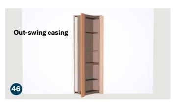
Position the left side casing. Test the door swing prior to screwing in to ensure it doesn't make contact with the floor.
