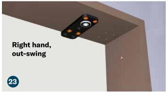
For a right-hand, out-swing door attach the upper jamb hinge (G) to the jamb top using (4) flat head Phillips sharp point 1" screws (K), lining up the hinge as shown. Make sure that you only use four screws. **DO NOT** drill into the two holes closest to the edge of the jamb as this can split your edge.
