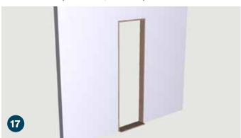
Place the door jamb into the rough opening. The bottom jamb threshold should extend into the room toward the back of the bookcase.
