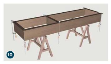
Place the bookcase onto saw horses, a work bench, or table. Place (6) wood clamps on the corners and the middle of the bookcase to secure the face frame while the glue dries.
