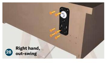
Match the bottom pivot hinge (J) to the pre-drilled holes at the bottom of the bookcase assembly as shown. With the plate lined up attach using (6) flat head Phillips sharp point 1" screws (K).
