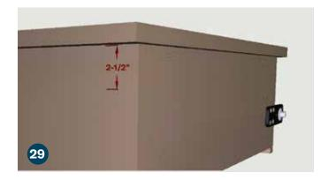
The friction door catch installs on the door side opposite the hinge. Make a mark 2-1/2 from the back of the door's face frame.
