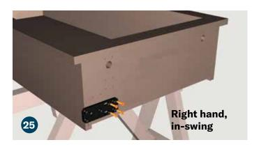
For a right hand, in-swing door line up the hinge as shown. Attach the top hinge plate (I) to the top bookcase assembly using (4) flat head Phillips sharp point 1" screws (K).
