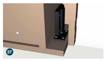
Now that the door assembly is in place use an adjustable wrench to tighten the carriage bolt just enough to catch the door catch.
