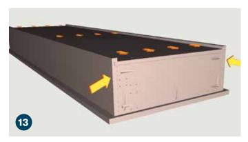
Ensure that the back is flush with the tops of the bookcase sides and that the bookcase is square. The pre-drilled holes on the back should align with the back bottom, back middle, and back top.
