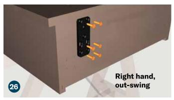
For a right hand, out-swing door line up the hinge as shown. Attach the top hinge plate (I) to the top bookcase assembly using (6) flat head Phillips sharp point 1" screws (K).
