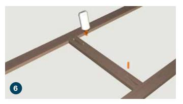
To install the front face frame turn the bookcase over. Add a small amount of wood glue to the dowel holes on the face frame assembly and insert (6) wooden dowels (C).
