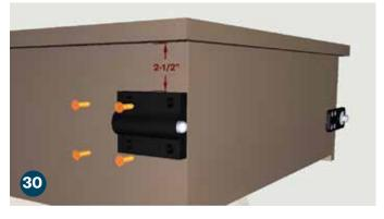
Position the friction door catch (M) at this mark, flush to the door bottom. Secure using (4) flat head Phillips sharp point 3/4" screws (L).
