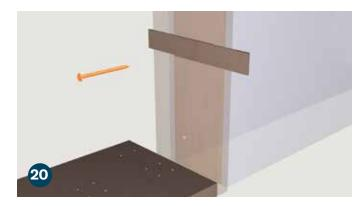
Using shims where needed, in stall (8) 3" jamb screws (F) making certain the top and sides of jamb are level.
