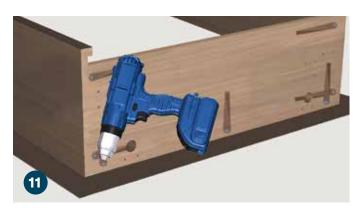
Remove wood clamps and flip the assembly over. Reinforce the top and bottom face frame with (6) 1" square head pocket screws (B).
