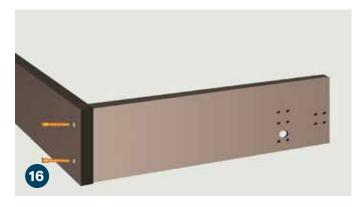
Position the jamb top making certain that the pre-drilled hinge holes are on the same side as jamb bottom hinge holes. After ensuring the corner is square; install (2)  $7 \times 50$ mm confirmat screws (E). Secure the remaining side jamb, making certain all corners are square, with (4)  $7 \times 50$ mm confirmat screws (E).
