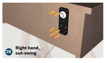
Match the bottom pivot hinge (J) to the pre-drilled holes at the bottom of the bookcase assembly as shown. With the plate lined up attach using (6) flat head Phillips sharp point 1" screws (K).
