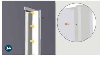
Secure the left casing to the face frame of the door using (5) 1-1/4" truss head screws (D). Make sure not to drill through other side of front casing.
