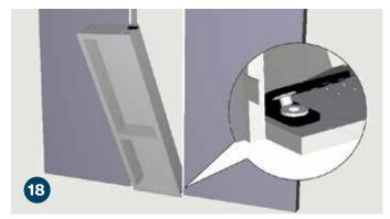
Place the door into the door jamb assembly. Ensure the bottom pivot hinge sits in the silver thrust bearing of the bottom jamb hinge.
