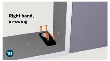
Align the holes in the bottom jamb hinge (H) with the predrilled holes in the jamb bottom threshold and attach using (5) flat head Phillips sharp point 1" screws (K).
