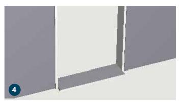
Place the door jamb assembly into the rough opening. The jamb bottom threshold should extend into the room toward the back of the bookcase.
