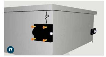
The friction door catch is installed on the door side opposite the hinge and flush to the bottom. Measure 2" from the back of the door face frame and make a mark. Position the friction door catch (M) at this mark, flush to the door bottom. Secure the catch using (4) flat head Phillips sharp point 3/4" screws (L).
