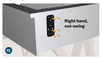
Align the top hinge plate (I) to the pre-drilled holes in the top bookcase assembly and attach using (6) flat head Phillips sharp point 1" screws (K).
