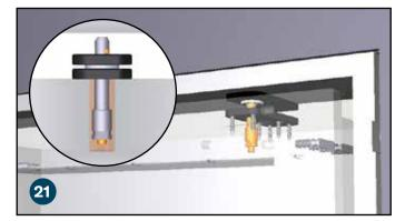
For an out-swing door the hinge pin inserts from the front side of the bookcase. Align the hole in the top of the bookcase with the hole in the top door hinge. Depress the hinge pin button and insert the hinge pin. The hinge pin will appear countersunk when properly installed and locked into place.
