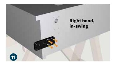
Align the holes in the top hinge plate (I) to the pre-drilled holes on the top bookcase assembly and attach using (4) flat head Phillips sharp point 1" screws (K).
