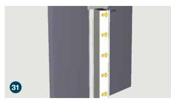
Using a 1/8" drill bit pre-drill five holes into the left support face frame. This will make it easier to attach the left side casing.
