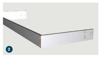
Position the jamb top ensuring that the pre-drilled hinge holes are on the same side as jamb bottom hinge holes. After ensuring the corners are square; attach the jamb top to the jamb side using (2) 7 x 50mm confirmat screws (E).
