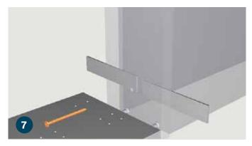
Using shims where needed, install (1) 3" jamb screws (F) making certain the top and sides of jamb are level.
