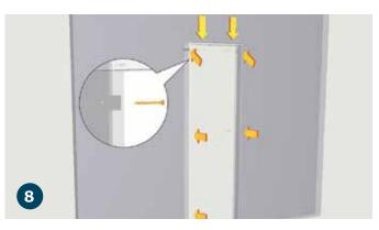
Using shims where needed, install (7) 3" jamb screws (F) making certain the top and sides of jamb are level.
