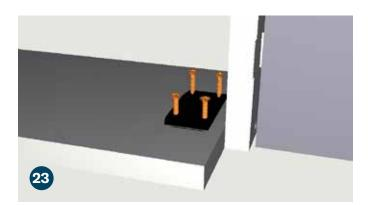
Remove the paper backing from the poly wedge and place it in the marked location. The wedge taper should face in for an in-swing door and out for an out-swing door. Secure with (4) flat head Phillips sharp point 3/4" screws (L).
