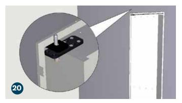
For an in-swing door, align the hole in the bookcase top hinge plate with the hole in the upper jamb hinge. Depress the hinge pin button and insert the hinge pin into the holes. Ensure that the pin locks into place.
