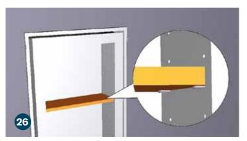
Slide the adjustable shelf into place onto the installed shelf pins. Repeat the previous step to insert the remaining adjustable shelves where desired.
