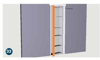
Position the left side casing. Test the door swing to ensure it does not contact the floor before securing the side casing with screws.
