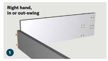
Align the jamb bottom threshold and (1) jamb side on a flat surface. The pre-drilled hinge holes on the jamb bottom threshold will be on the right for a right hand in or out-swing, on the left for a left hand in or out-swing. After ensuring the corner is square; attach the jamb bottom threshold to the jamb side using (2) 7 x 50mm confirmat screws (E).
