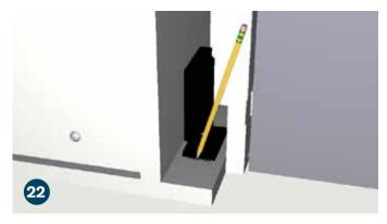
Place the poly wedge (O) where the doorstop carriage bolt will go when the door is closed. Ensure that the door is flush. Mark out the poly wedge location with a pencil or tape.
