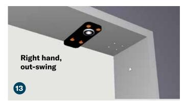
For a right-hand, out-swing door align the holes in the upper jamb hinge (G) to the pre-drilled holes in the jamb top and attach using (4) flat head Phillips sharp point 1" screws (K). Make sure that you only use four screws. **DO NOT** drill into the two holes closest to the edge of the jamb as this can split your edge.
