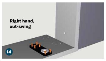
Align the bottom jamb hinge (H) to the pre-drilled holes in the jamb bottom threshold and attach using (6) flat head Phillips sharp point 1" screws (K).
