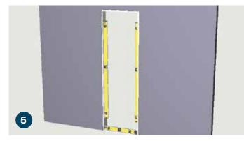
It is critical that the jamb bottom threshold and jamb sides are level. If the door jamb assembly is not level and plumb the door will not swing and close properly.
