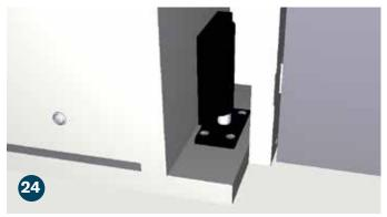
Now that the door assembly is in place use an adjustable wrench to tighten the carriage bolt just enough to catch the poly wedge.
