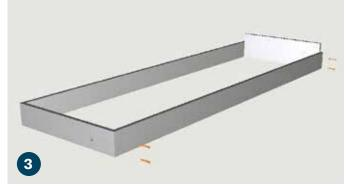
Align the remaining side jamb to the assembly, ensuring all corners are square, and attach it using (4)  $7 \times 50$ mm confirmat screws (E).
