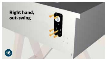
Align the holes in the bottom pivot hinge (J) to the pre-drilled holes at the bottom of the bookcase assembly and attach using (6) flat head Phillips sharp point 1" screws (K).
