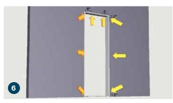
Using a 1/8" drill bit, pre-drill and countersink three holes into each of the jamb sides 2" from the top, 2" from the bottom, and in the middle.
