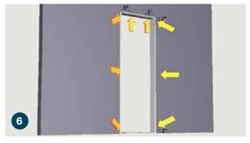
Using a 1/8" drill bit, pre-drill and countersink three holes into each of the jamb sides 2" from the top, 2" from the bottom, and in the middle.
