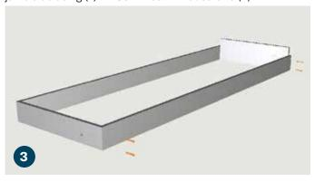
Align the remaining side jamb to the assembly, ensuring all corners are square, and attach it using (4)  $7 \times 50$ mm confirmat screws (E).
