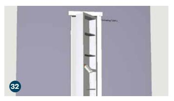
Run a bead of glue down the face frame of the door to strengthen the left casing.
