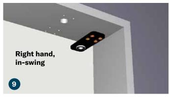
To install a right hand, in-swing door align the holes in the upper jamb hinge (G) with the pre-drilled holes in the jamb top and attach using (4) flat head Phillips sharp point 1" screws (K). For a left hand door use the same pre-drilled hole on the opposite side for all hinge placement.
