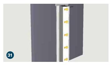
Using a 1/8" drill bit pre-drill five holes into the left support face frame. This will make it easier to attach the left side casing.
