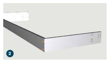
Position the jamb top ensuring that the pre-drilled hinge holes are on the same side as jamb bottom hinge holes. After ensuring the corners are square; attach the jamb top to the jamb side using (2)  $7 \times 50$ mm confirmat screws (E).
