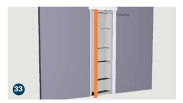
Position the left side casing. Test the door swing to ensure it does not contact the floor before securing the side casing with screws.
