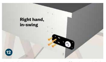
Align the holes in the bottom pivot hinge (J) to the pre-drilled holes at the bottom of the bookcase assembly and attach using (4) flat head Phillips sharp point 1" screws (K).
