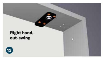
For a right-hand, out-swing door align the holes in the upper jamb hinge (G) to the pre-drilled holes in the jamb top and attach using (4) flat head Phillips sharp point 1" screws (K). Make sure that you only use four screws. **DO NOT** drill into the two holes closest to the edge of the jamb as this can split your edge.
