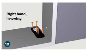
Align the holes in the bottom jamb hinge (H) with the predrilled holes in the jamb bottom threshold and attach using (5) flat head Phillips sharp point 1" screws (K).
