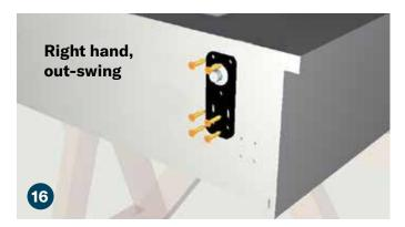
Align the holes in the bottom pivot hinge (J) to the pre-drilled holes at the bottom of the bookcase assembly and attach using (6) flat head Phillips sharp point 1" screws (K).
