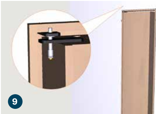
9 Align the holes of the bookcase top jamb hinge and the top door hinge. Depress the hinge pin button and insert making certain that it locks into place. On an out-swing door the pin will insert from the front of the bookcase and appear countersunk when properly locked.
