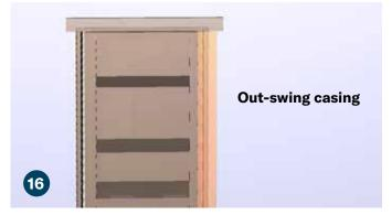
Attach the right casing onto the door jamb with a 1/2" overhang on the door face frame.
