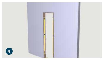
It is critical that the bottom threshold and jamb sides are level. If the door jamb is not level and plumb the door will not swing and close properly.
