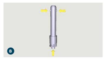
Press down on the ball lock of the hinge pin to retract the two top pins.
