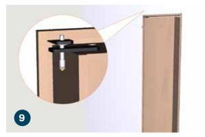
Align the holes of the bookcase top jamb hinge and the top door hinge. Depress the hinge pin button and insert making certain that it locks into place. On an out-swing door the pin will insert from the front of the bookcase and appear countersunk when properly locked.
