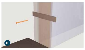
Using shims where needed, install (8) 3" jamb screws (F) making certain the top and sides of the jamb are level.
