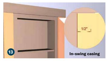
Position the right and left side casings with a 1/2" overhang on the face frame of the door. Attach using a brad nailer.
