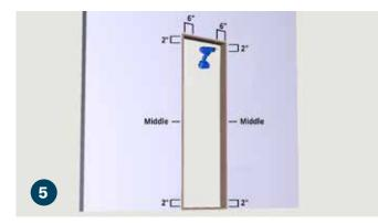
Using a 1/8" drill bit, pre-drill and countersink three holes into each side of the jamb, 2" from the top of the jamb, 2" from the bottom of the jamb, and in the middle. Next pre-drill and countersink two holes into the jamb top, 6" from the right and left sides of the jamb.
