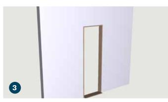
Place the door jamb into the rough opening. The bottom jamb threshold should extend into the room toward the back of the bookcase.
