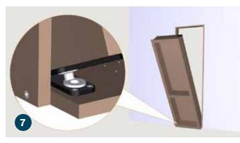
Place the door into the door jamb, making sure that the bottom pivot hinge sits in the silver thrust bearing.
