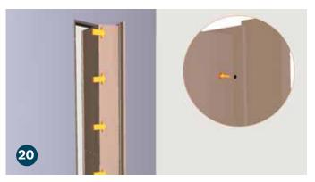
Secure with (5) 1-1/4" truss head screws (D) making sure not to drill through other side of front casing.
