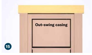
For an out-swing door, center the top casing over the door leaving a 1/16" clearance over the door itself. Attach using a brad nailer.
