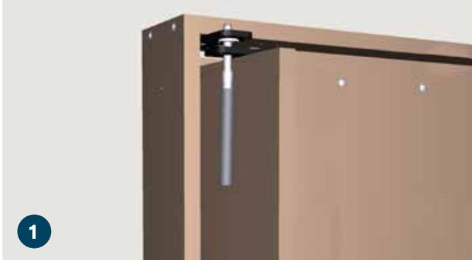
Locate the hinge in the upper corner of the door. Place the hinge pin removal tool (Q) on the hinge pin to retract and pull down as shown. On an out-swing door the hinge pin will be countersunk inside of the bookcase.
