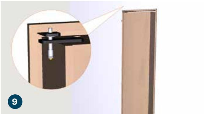
9 Align the holes of the bookcase top jamb hinge and the top door hinge. Depress the hinge pin button and insert making certain that it locks into place. On an out-swing door the pin will insert from the front of the bookcase and appear countersunk when properly locked.
