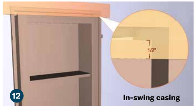
12 For an in-swing door, position the top casing with a 1/2" overhang on the face frame of your door. Attach using a brad nailer.
