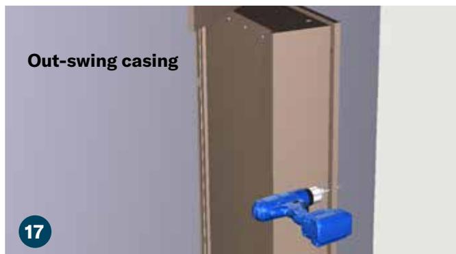
Using a 1/8" drill bit pre-drill and countersink five holes into the left support face frame. This will make it easier to attach the left side casing.
