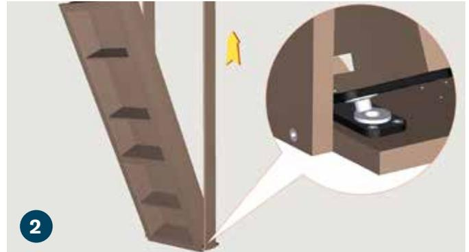
Remove the door from the jamb by lifting it up and off the bottom jamb hinge.
