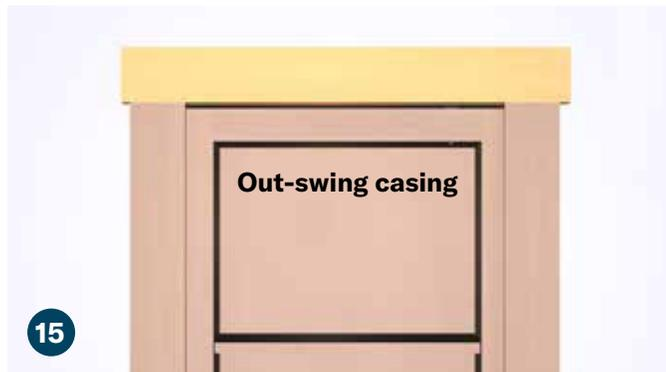
For an out-swing door, center the top casing over the door leaving a 1/16" clearance over the door itself. Attach using a brad nailer.
