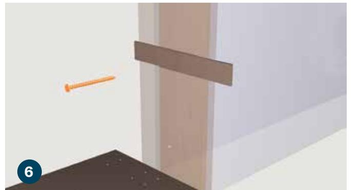
Using shims where needed, install (8) 3" jamb screws (F) making certain the top and sides of the jamb are level.
