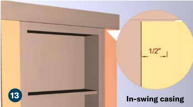
Position the right and left side casings with a 1/2" overhang on the face frame of the door. Attach using a brad nailer.
