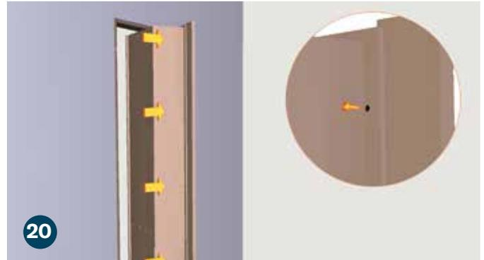
Secure with (5) 1-1/4" truss head screws (D) making sure not to drill through other side of front casing.
