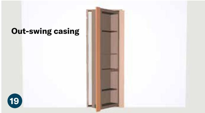
Position and attach the left side casing. Test the door swing prior to screwing in to ensure it doesn't make contact with the floor.
