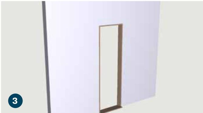
Place the door jamb into the rough opening. The bottom jamb threshold should extend into the room toward the back of the bookcase.
