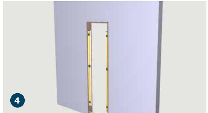
It is critical that the bottom threshold and jamb sides are level. If the door jamb is not level and plumb the door will not swing and close properly.
