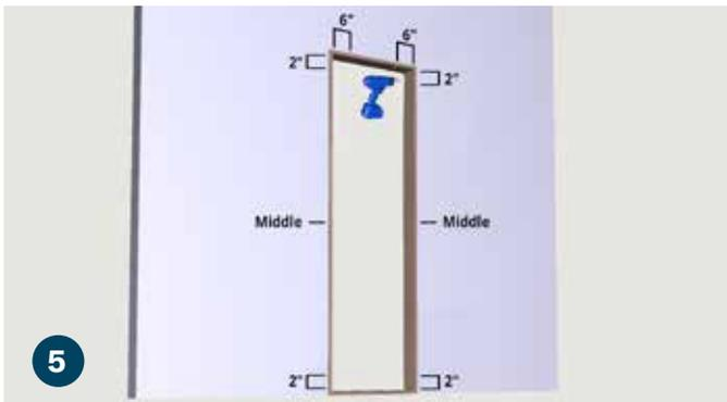
Using a 1/8" drill bit, pre-drill and countersink three holes into each side of the jamb, 2" from the top of the jamb, 2" from the bottom of the jamb, and in the middle. Next pre-drill and countersink two holes into the jamb top, 6" from the right and left sides of the jamb.
