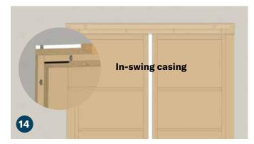
Align the clips in the top casing the same way you did the side and press firmly into place. Adjust the top and side casing until they sit flush against each other and are square.
