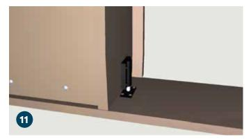
With the door assembly in place, tighten the carriage bolt with an adjustable wrench just enough to catch on the poly wedge. Repeat steps 7 - 11 to install the second bookcase carriage.
