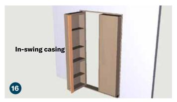
Run a bead of glue down the face frame side, avoiding drilled holes. Position the center casing and firmly press into place.
