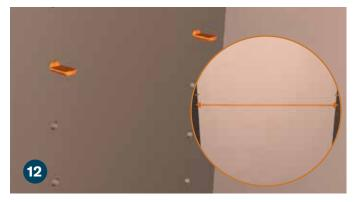
Add (2) shelf pins (P) where desired and (2) shelf pins directly across from them. Slide the shelf into place onto the installed shelf pins. Do the same for the remaining shelves as desired.
