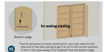
Align the clips in the side casing and on the jamb. Press firmly into place. The bottom edge of each piece of side casing is indicated with a small, drilled hole on the back side near the bottom clip pocket. The clip pockets will be closer to the inner edge of the casing. The top of the side casings should sit about 1/2" below the top of the door. If it is higher than this firmly grip the side casing and slide it down until it stops.
