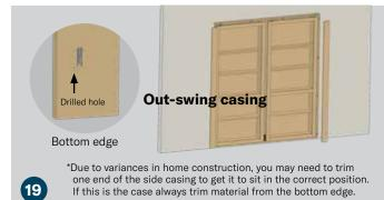
Align the clips in the side casing and on the jamb. Press firmly into place. The bottom edge of each piece of side casing is indicated with a small, drilled hole on the back side near the bottom clip pocket. The clip pockets will be closer to the inner edge of the casing. The top of the side casings should sit about 1/16" above the top of the door. If it is higher than this firmly grip the side casing and slide it down until it stops.
