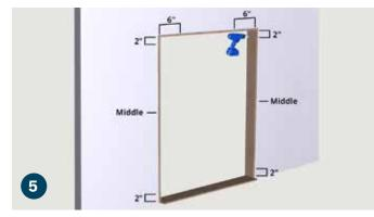
Using a 1/8" drill bit pre-drill and countersink three holes into each side of the door jamb, 2" from the top of the jamb, 2" from the bottom of the jamb, and in the middle. Next pre-drill and countersink two holes into the jamb top, 6" from the right and left sides of the jamb.
