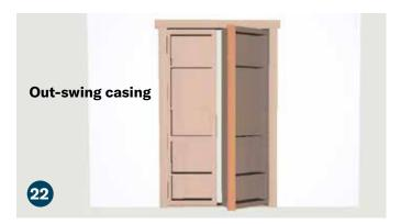
Run a bead of glue down the face frame of the door, avoiding the drilled holes, to strengthen the center casing. Firmly press the center casing into place. Test the door swing prior to screwing in to ensure it doesn't make contact with the floor.
