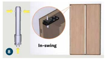
Press down the ball lock of the hinge pin (N) to retract the (2) top pins. Align the holes of the top jamb hinge and top hinge plate and insert the pin making certain it locks into place. Repeat to install the second bookcase assembly. The hinge pins installs from the front of the bookcase on an out-swing door and will appear countersunk when properly installed and locked into place.
