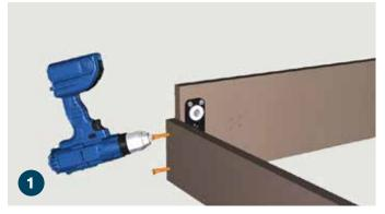
Align the jamb bottom threshold and (1) jamb side on a flat surface. Be certain that they sit flush at the front and that the pre-installed hinges face in. After ensuring that the corner is square pre-drill, countersink, and install (2) 7 x 50mm confirmat screws (E).
