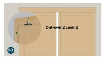
Align the clips in the top casing the same way you did the side and press firmly into place. Adjust the top and side casing until they sit flush against each other and the gap between the top casing and the top of the door is uniform.
