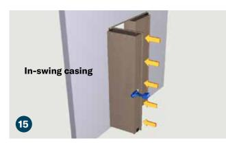
Using a 1/8" drill bit pre-drill five holes into either the left face frame side of the right bookcase or the right face frame side of the left bookcase. The center casing will be attached to whichever frame side you have drilled.
