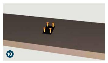
Remove the sticker from the back of the poly wedge and place in the marked location. The wedge tapers should face in for an in-swing door and out for an out-swing door. Secure with (4) Flat Head Phillips Sharp Point 3/4" Screws (L).
