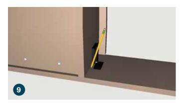
Place the poly wedges (O) where the friction catch carriage bolt will go when the door is closed. Ensure that the door is flush. Mark the location with a pencil or tape.
