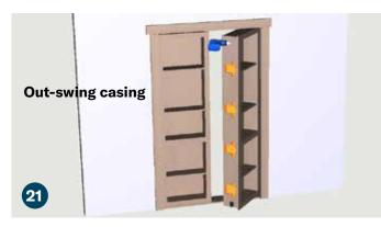
Using a 1/8" drill bit pre-drill and countersink five holes into either the left face frame side of the right bookcase or the right face frame side of the left bookcase. The center casing will be attached to whichever frame side you have drilled.
