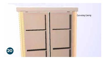
Position the left and right side casings with a 1/2" overhang on the face frame of the door. Attach using a brad nailer.
