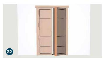
Run a bead of glue down the face frame of the door, avoiding the drilled holes, to strengthen the center casing. Firmly press the center casing into place. Test the door swing prior to screwing in to ensure it doesn't make contact with the floor.
