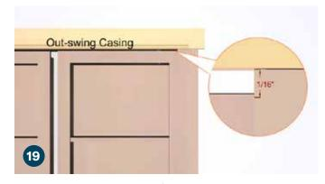
Center the top casing with a 1/16" clearance over the doors. Attach with a brad nailer.
