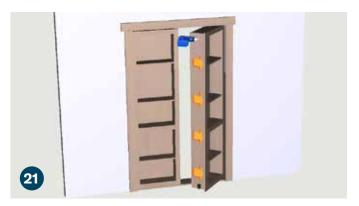
Using a 1/8" drill bit pre-drill and countersink five holes into either the left face frame side of the right bookcase or the right face frame side of the left bookcase. The center casing will be attached to whichever frame side you have drilled.
