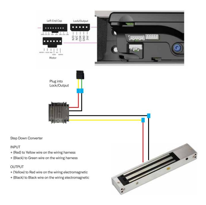
**NOTE:** Additional 18 gauge wire will be needed for installation.
