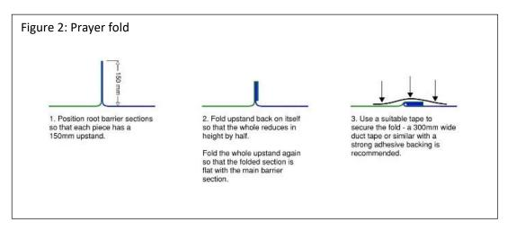
Installation and jointing must always follow manufacturer's guidance. Both welded and taped joints should be completed in dry conditions.
