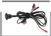
Emulation/acquisition cable, with PWM power generator function such as PWM POWER with integrated 5V voltage generator; mass generator and control of the Feedback. It is used for the activation of feedback controlled components via potentiometers
