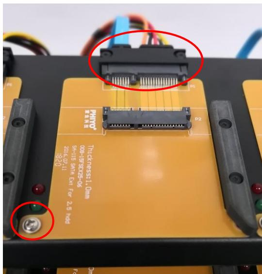
Step 2. Unplug the original adapter board and replace it with a new one.
