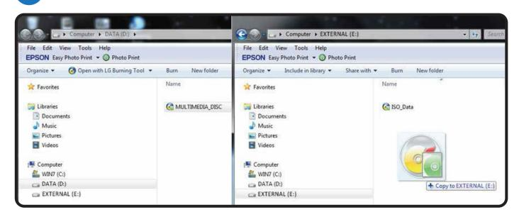
After the ISO file is transferred to the duplicator's HDD, please turn the USB switch OFF and reboot the duplicator.
