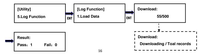
Open the file from computer. The file name of log file is "LOG\_DATA\_XXXX.txt". XXXX is from 0000 to 9999 in sequence. If no log file in the disk, it starts from 0000. If 0000 is exist in the disk, it will be added 1 to be 0001 and so on. The information in log file is shown below. It was recorded for 1 to 3 Disk to Disk Copy and uses 5 log records.
