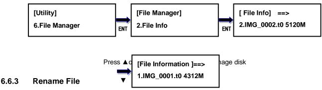
Rename the file instead of using default file names (IMG\_0001, IMG\_0002, etc.). Only needs to rename the file IMG\_XXXX.t0, the file IMG\_XXXX.dd will be renamed as the IMG\_XXXX.t0 automatically.
