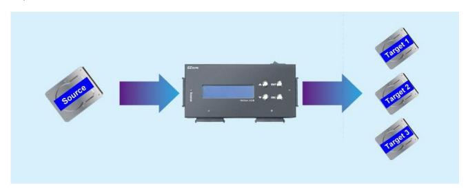
**Disk to File** Images the source disk to a file and stores in a large image disc. The different image files can be stored in a large image disc in sequence. Images HDD 1 then HDD 2 and then HDD 3.
