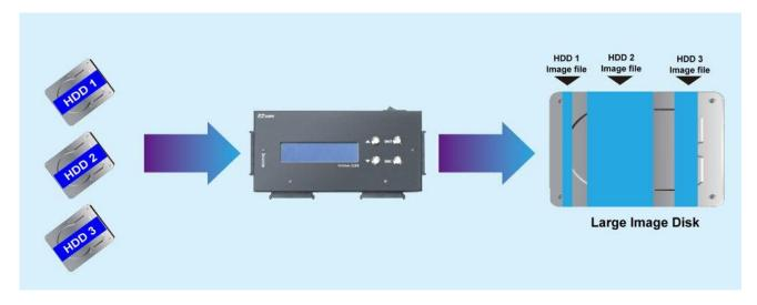
**File to Disk** Restores image file from a large image disc to target disks. Users can choose one of the image file in the large image disc to be restored. Up to 3 target disks can be restored at
