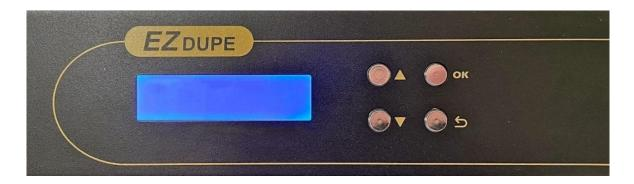
**▲ Button:** *Up, Backward:* To navigate backward in the menu. **▼ Button:** *Down, Forward:* To navigate forward in the menu.
