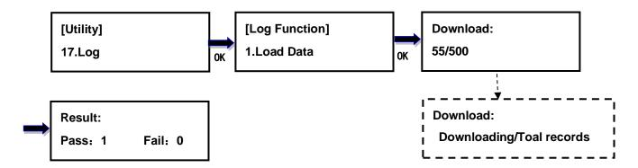
Open the file from computer. The file name of log file is "LOG\_DATA\_XXXX.txt". XXXX is from 0000 to 9999 in sequence. If no log file in the disk, it starts from 0000. If 0000 is exist in the disk, it will be added 1 to be 0001 and so on. The information in log file is shown below. It was recorded for 1 to 3 Copy and uses 5 log records.
