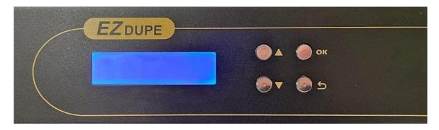
▲Button: <u>Up, Backward</u>: To navigate backward in the menu. ▼Button: <u>Down, Forward</u>: To navigate forward in the menu.
