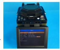
darkness. The fiber fusion splicer can provide fine imaging system and its advanced digital design makes the image display exquisite and clear. The embedded real-time operating system provides a friendly interface and abundant functionality. The built-in super capacity of a long time high performance lithium battery offers reliable field work.
