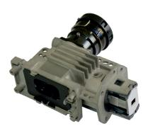
STAR CORE is a compact optics designed for the TI DLP® chip up to 0.7" diameter, orthogonal pixel architecture, and 12° tilt angle. The DLP chip illumination is well homogenous thanks to an integrator rod that acts as a convenient light input port.\*
