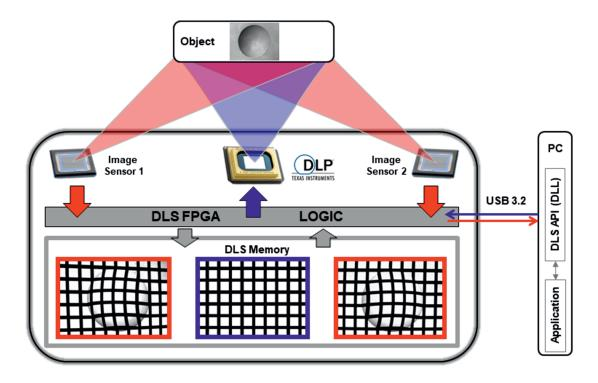
A sequence of user-defined projection patterns is uploaded into the DLS memory (RAM) and the data can be used for a single projection or for a projection loop. The illuminated object is recorded by the sensors and the images are buffered in the on-board RAM that holds up to 1.592 pictures (10 bit, 1.920 x 1.200 pixels), ready for download to the PC for further processing. All data flow operations are executed by one FPGA device enabling the outstanding real-time precision.
