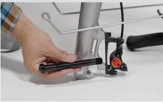
Remove brake pad spacer from in between brake pads - it may be tight but simply pulls out. If this piece is not in place, skip this step.
