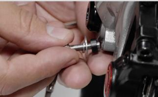
Make sure to install washer and spacer as shown.
