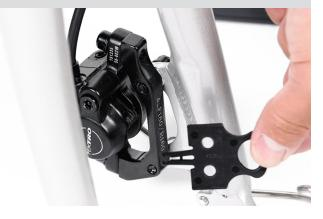
Lift the fork, place the wheel partially in the fork, then line up the brake rotor between the pads and mount the wheel fully into the fork.
