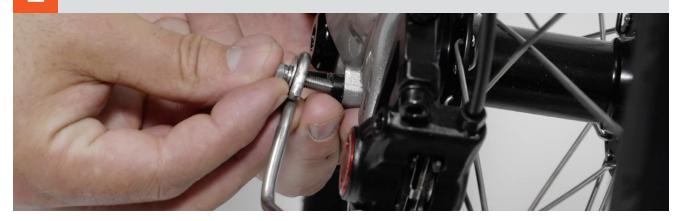
Tighten fender support strut hardware.
