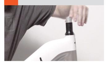
Mount stem on fork, lift rubber cover, drop bolt from Step 2 into stem, and tighten until so that spacers no longer rotate.
