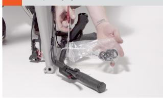
Use a 5mm allen wrench to remove the top bolt from the fork, along with the black top cap. Set aside the top cap, you will not need it.
