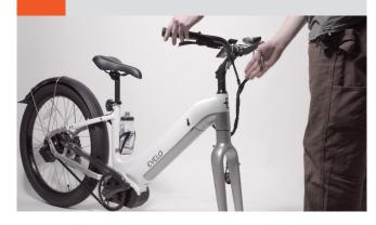
Use a 4mm allen wrench to tighten both bolts on the side of the stem.
