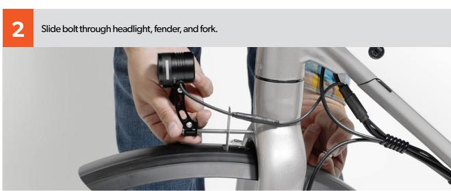
Attach headlight and fender assembly to fork. Position the fender as high up as possible and tighten the bolt and nut.
