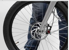
Slide the thru-axle into the fork and wheel and securely tighten with an allen wrench.
