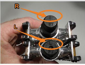
It is important to note that the pedals are threaded differently. The right pedal screws in clockwise and the left pedal screws in counter-clockwise.
