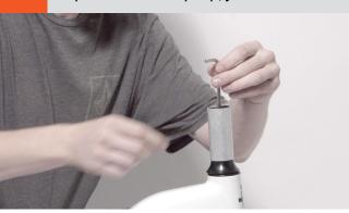
Remove silver spacer from fork and install black headset spacers from Step 1.
