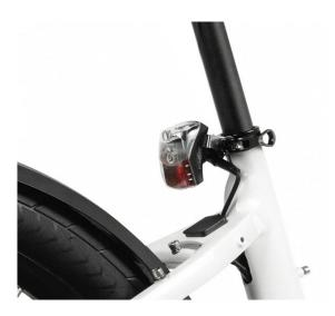
**Step 1:** Open the seatpost quick release, then unscrew it to remove the light. Unplug the connector, then reassemble and tighten the seatpost quick release.
