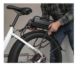
**Step 3:** Remove the battery from the rack and hold the rack in place on the bike.
