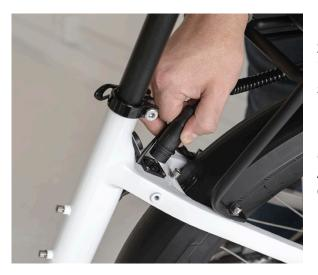
**Step 7:** Open the cover and plug the battery into the frame port. It should only go in one way, so be aware of the plug orientation.
