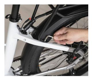
**Step 5:** Using an allen wrench, install the upper mounting bolts. Use the longer bolts from the rack package; the bolts that came on the bike are too short to hold the rack securely.
