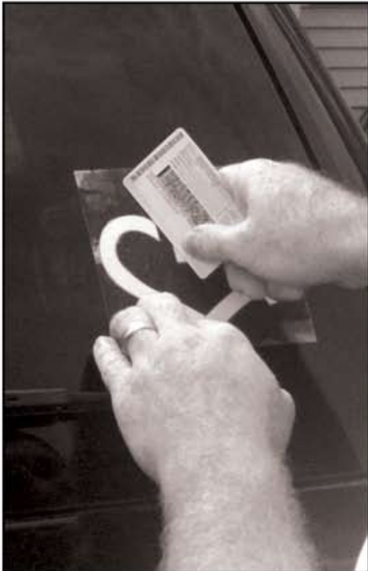
4. USE HARD EDGE (CREDIT CARD/LICENSE WILL WORK) TO FLATTEN; RUB VINYL DECAL ONTO VEHICLE
