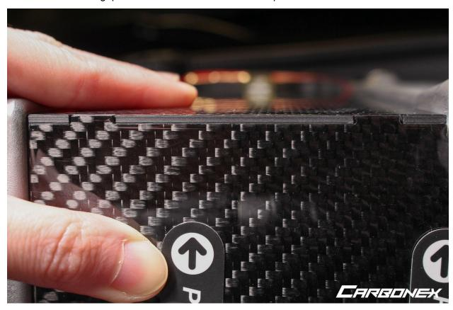
5. WARNING: For the following steps, please apply constant pressure in the direction of the green arrows to ensure the alignment tabs stay locked in and there are no gaps until the installation is complete.
