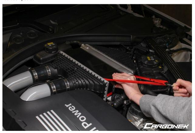
10. Continue to apply pressure to the smaller intercooler cover, and slowly pull one of the guided installation stickers in the upward direction. **Note: always pull slowly to ensure** the 3M red backing tape does not get over stretched and torn.
