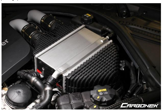
3. Place the larger intercooler cover on top of the intercooler with the guided sticker (PULL) arrow pointing towards the front of the car
