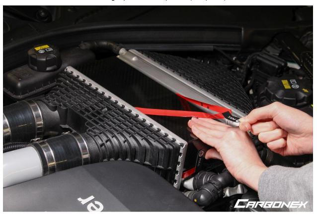
8. Apply light pressure on the back of the intercooler cover to bond the 3M double sided tape and secure the intercooler cover to the OEM intercooler.
