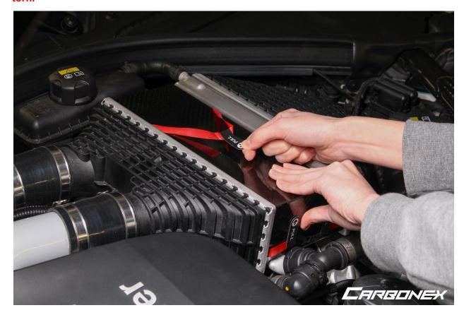
7. Pull until half of the 3M red backing tape has been pealed (see photo)
