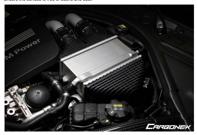
2. Place the smaller intercooler cover vertically with the guided stickers (PULL) arrows pointing up
