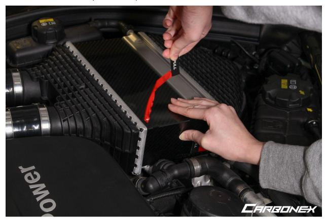
13. Continue to apply pressure to the smaller intercooler cover, and slowly pull the other guided installation stickers in the upward direction. **Note: always pull slowly to ensure the 3M red backing tape does not get over stretched and torn.**
