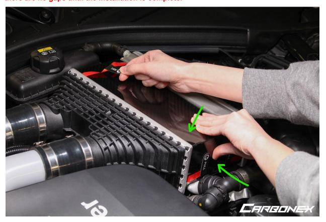
6. Slowly pull the guided installation sticker towards the front of the vehicle. **Note: always** pull slowly to ensure the 3M red backing tape does not get over stretched and torn.
