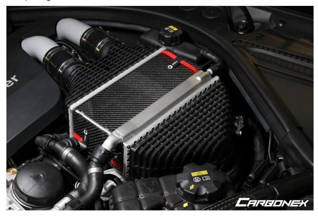
4. Bring the 2 intercooler covers towards each other until the alignment tabs meet and form a 90 degree angle.
