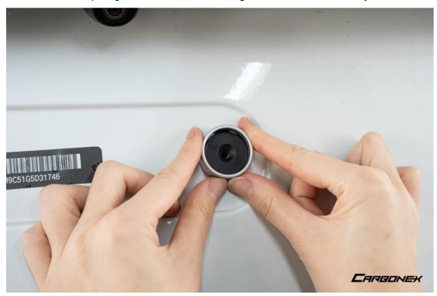
7. Secure the trunk magnet with the trunk magnet screw. Please ensure the threads are aligned before applying force to avoid stripping the nylon nut.
