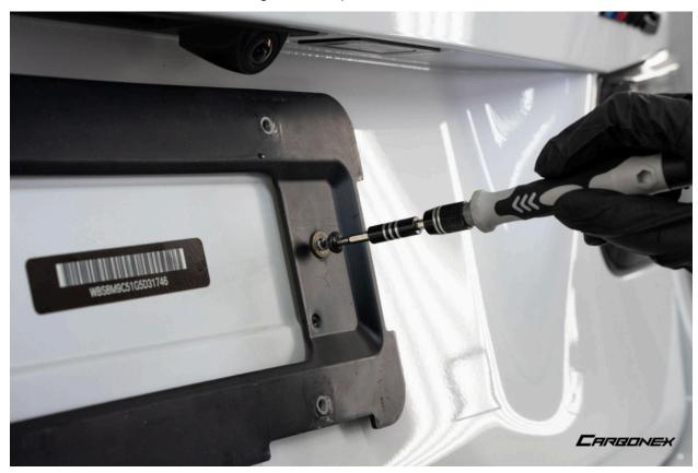
3. Before proceeding any further, please ensure your vehicle has the nylon nut on the trunk similar to ones in the photo. If this is not the case, the plate mount might not be compatible with your vehicle, please contact our customer service at <a href="mailto:info@carbonexauto.com">info@carbonexauto.com</a>.
