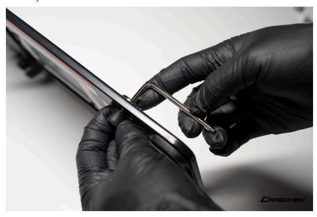
28. Align the license plate assembly with the trunk magnet, the mounts and magnets are designed for easy alignment and they should simply click in place.
