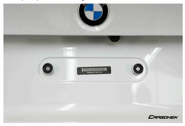
The next step is to determine if 2 or 4 bolts will be used to mount your license plate. We recommend using 4 bolts to avoid rattling when closing your trunk.
