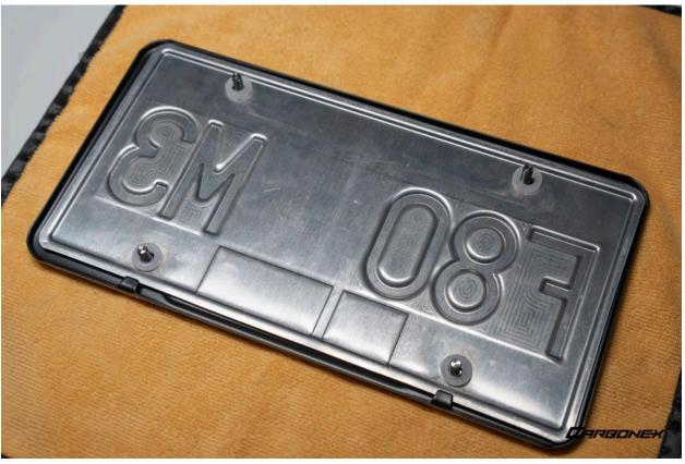
12. Install the plate mount assembly with the warning sticker facing upwards.
