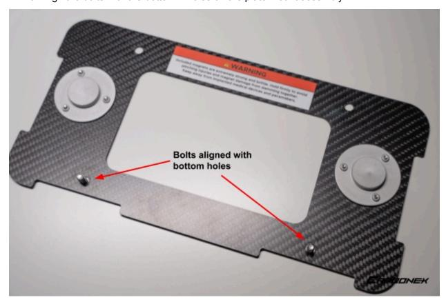
20. Hand tighten 2 rubberized nuts onto the bolts
