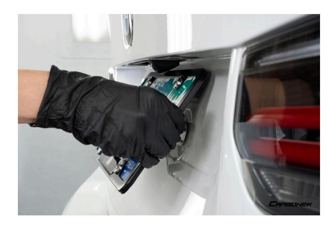
16. Ensure both aluminum magnet mounts are fully engaged and the 4 rubberized nuts are contacting the trunk
