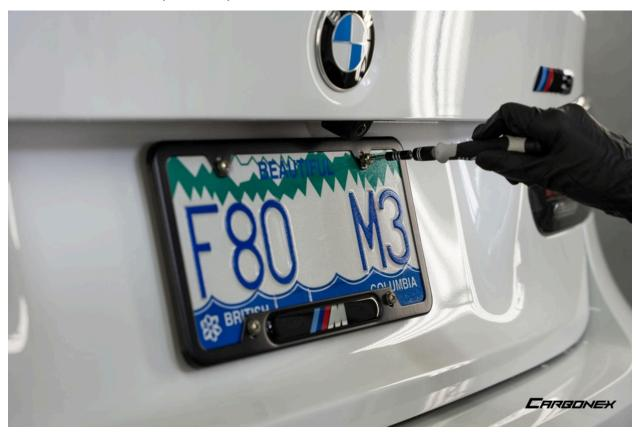
2. Remove two screws securing the OEM plate mount to the trunk
