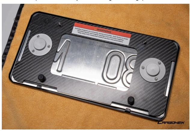
26. Hand tighten 2 rubberized nuts onto the bolts
