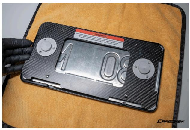
13. Hand tighten the 4 rubberized nuts onto the bolts
