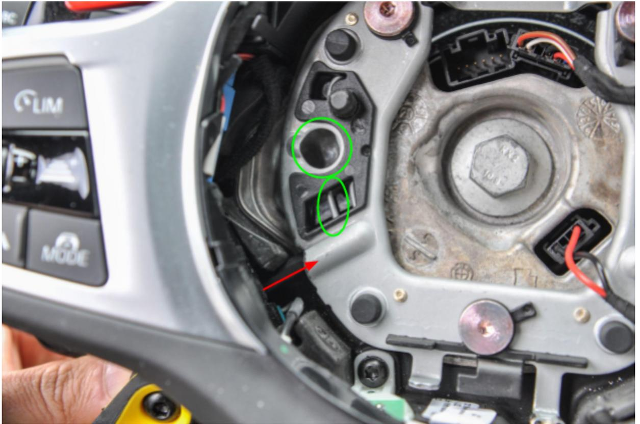
3. Once the airbag is loose, carefully disconnect the airbag connector to the steering column and set aside the airbag in a safe place.
