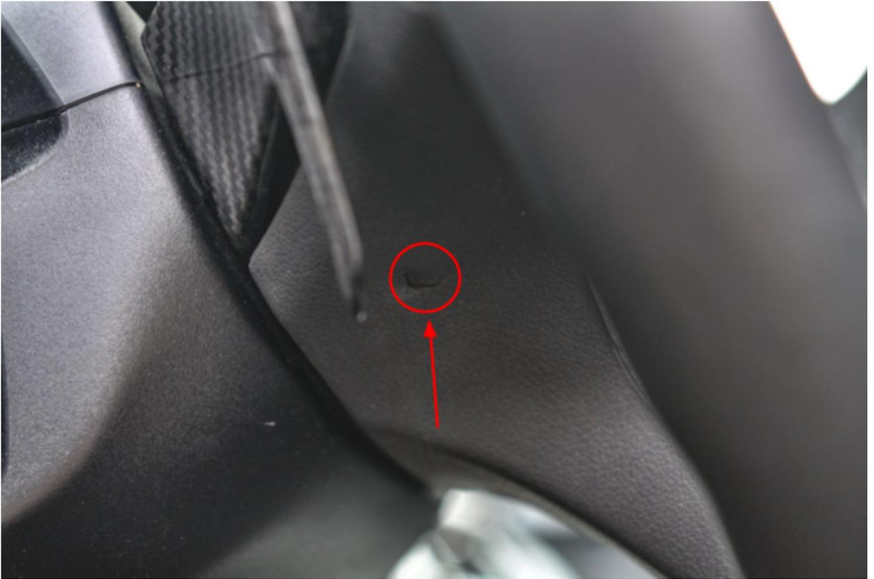
The image below is the internal structure behind the airbag (you won't see this until the airbag is removed). The screwdriver is pressing on the silver retaining clip in the direction indicated by the red arrow. Once compressed, the retaining clip at the red circle area will be fully compressed and out of the way, letting the airbag come free
