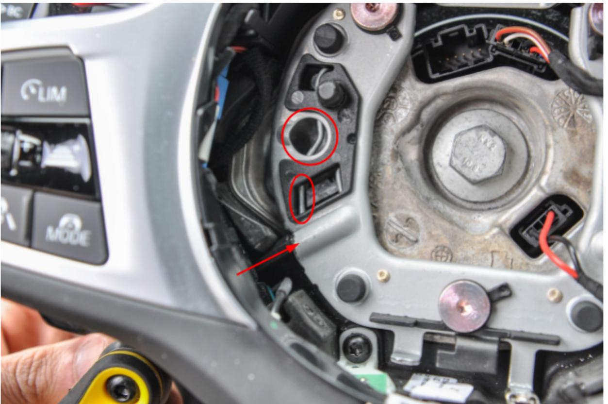
This image below shows the retaining clip compressed by the screwdriver, notice the clip in the top green circle has been fully compressed and the airbag is able to come loose.
