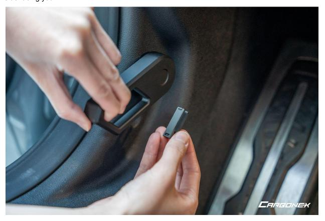
10. Gently insert the pin into the hood latch handle. You should hear a click when the pin is fully inserted.
