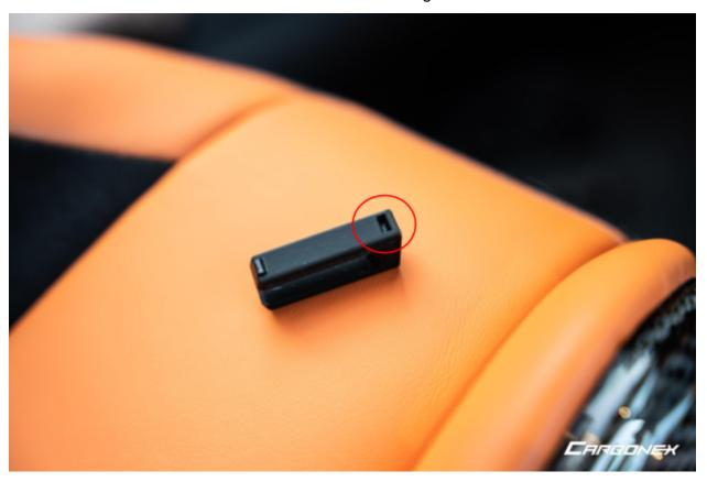
9. Pull the Carbonex hood latch handle to the full extent and take this pin with the slotted side facing you
