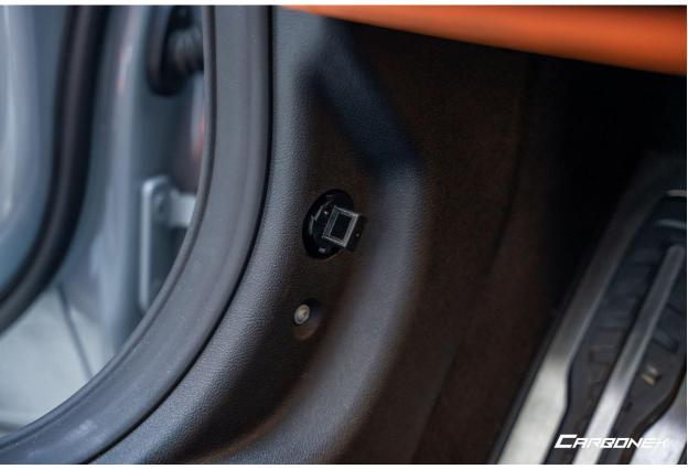
6. Take the Carbonex hood latch handle and make sure all mounting points are aligned
