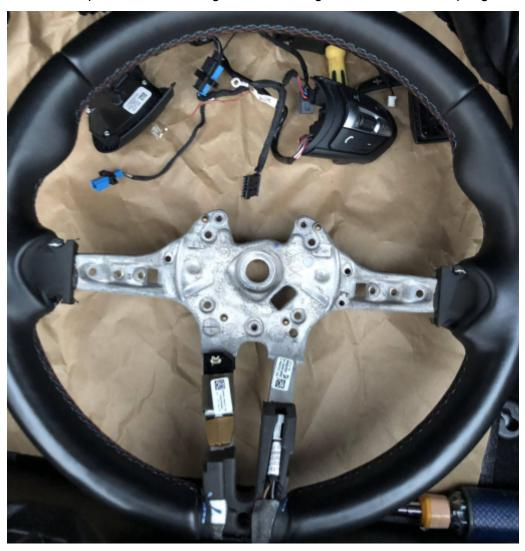
17. Turn the wheel over again and undo the metal clips on the lane departure vibration motor. The way to remove these is by pressing hard on the bracket in the direction of the red arrow. Simultaneously, use a flat head screwdriver to undo the clip.
