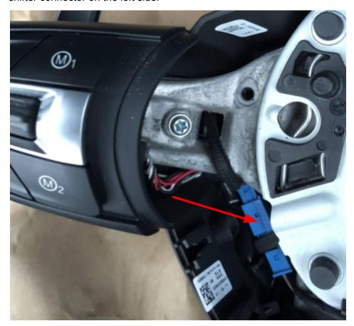
15. The blue paddle shifter connector on the right side is beneath the cruise control module, which can be removed by simply sliding it out of the plastic back housing. Disconnect the blue connector.
