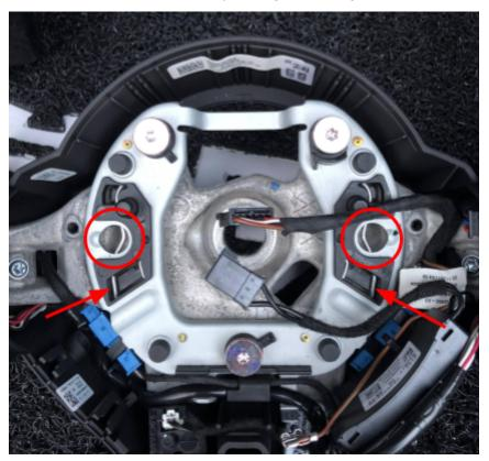
3. Once the airbag is loose, carefully disconnect the 3 connectors to the steering column and set aside the airbag in a safe place.
