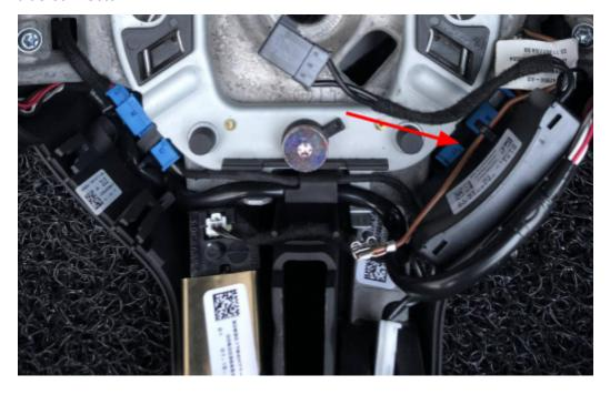
16. Remove the plastic back housing, buttons, wiring harness, and horn springs.
