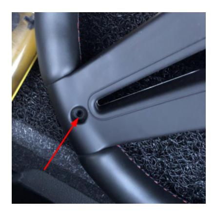
7. Undo the 2 clips near the bottom of each side and 3 clips at the top with a trim tool. Once the clips are undone, the trim can be removed from the steering wheel.
