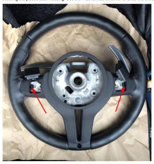
14. Turn the steering wheel over back to the front side and disconnect the blue paddle shifter connector on the left side.
