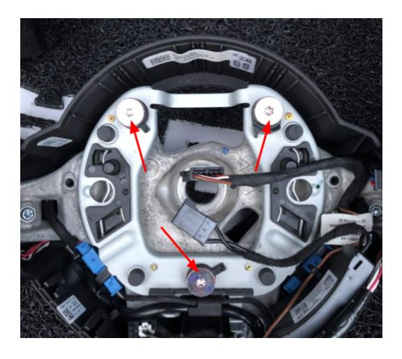
9. Use the T-20 torx screwdriver, remove the ground screw.
