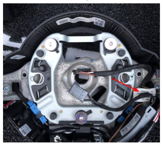
10. Disconnect the lane departure vibration motor cable and the ground cable.
