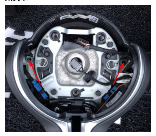
6. Flip the steering wheel over and use the T-20 torx screwdriver to remove the screw securing the back of the steering wheel trim at the 6 o'clock position.
