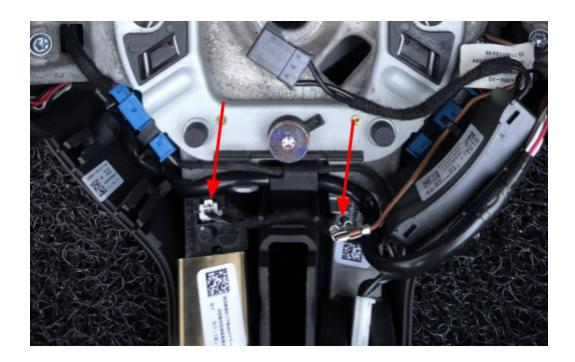
11. Starting on the left side, use the T-20 torx screwdriver to remove the screw securing the paddle shifters. Once done, do the same for the paddle shifter on the right side.
