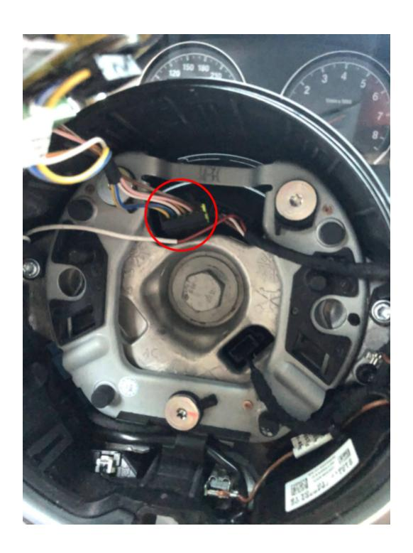
4. Starting on the left side, use the T-20 torx screwdriver to remove the screw securing the paddle shifters. Once done, do the same for the paddle shifter on the right side.
