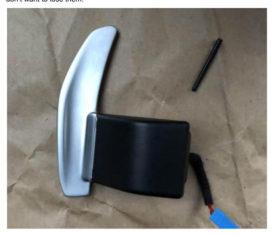
8. Carefully lift the paddle shifters on the side where the pin was removed and slide the paddle shifters off the latches to remove completely. Be very careful to not lose the spring and the plastic "bridge" piece marked in the second image.
