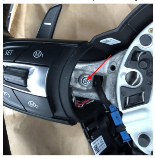
5. The photos from this step onwards have the paddle shifter removed to better illustrate the replacement process but the paddle shifter module does not need to be removed to replace the paddle shifters. Start on one side, pull the paddle shifters back (away from the steering wheel) and you should be able to see the pin securing the top and bottom halves of the paddle shifter module.
