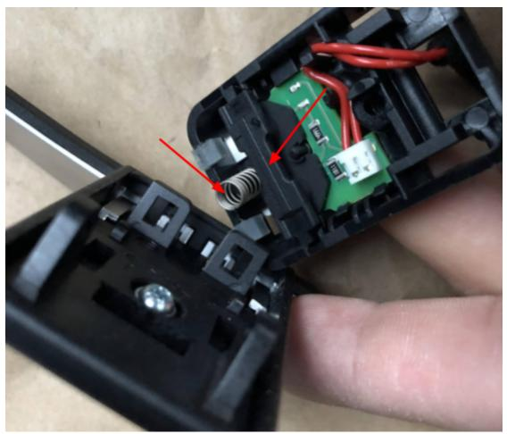
9. Remove the T-15 torx screw securing the paddle shifters to the plastic back housing
