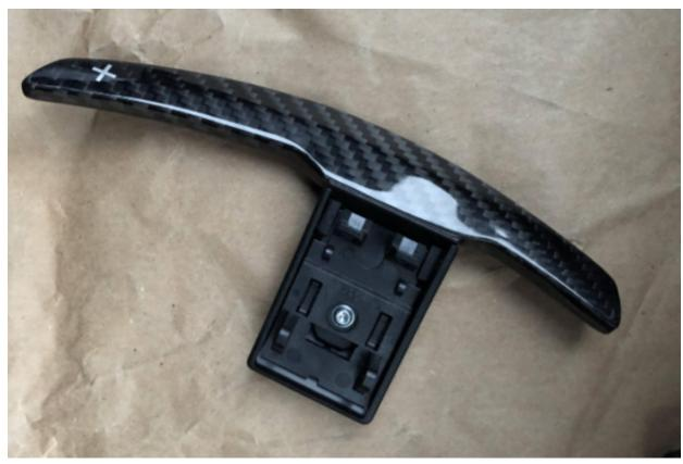
13. Reinstall the new paddle shifters back onto the paddle shifter module, reinsert the pin to secure in place.
