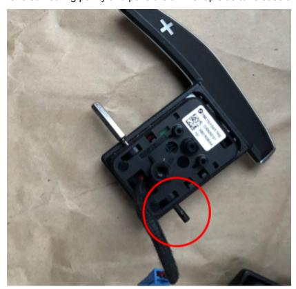
7. Remove the pin and orient the paddle shifters in such a way that the back of the paddle shifters is facing upward (parallel to the roof of the vehicle). This is to ensure when disassembling the paddle shifter module, the internal components don't fall out as you don't want to lose them.
