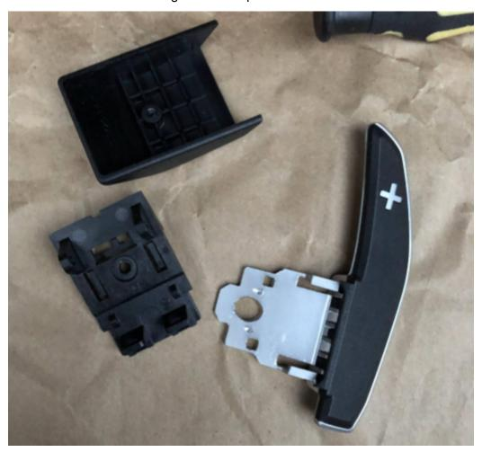
12. Install the plastic bracket onto the new paddle shifters and secure the plastic back housing with the T-15 torx screw.
