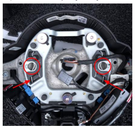
3. Once the airbag is loose, carefully disconnect the airbag connector to the steering column and set aside the airbag in a safe place.
