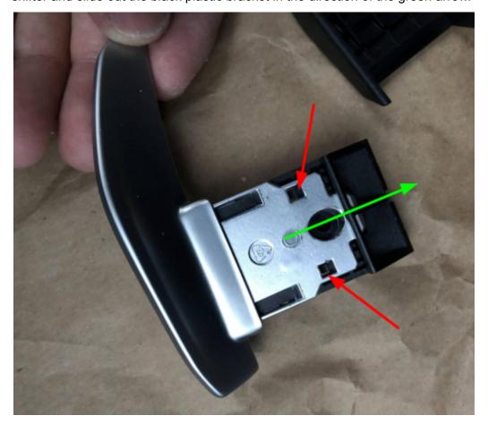
11. You should now have all the components disassembled and ready to transfer the plastic bracket and the back housing to the new paddle shifters.
