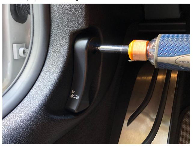
2. Remove the OEM hood latch handle and install the Carbonex billet hood latch handle.
