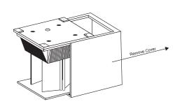
Remove the outside cover from the main body of the wall lamp.
