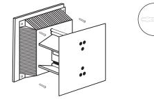
2 Use the screwdriver to remove the base of the lamp from the main body.
