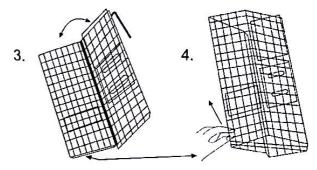
Flip the cage over to the right hand side and then lift the cage up.
