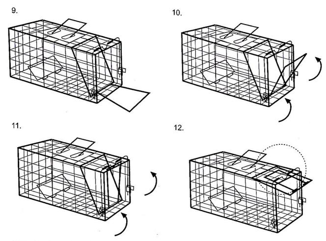
Lift the trap door spring and push towards the bait plate. Now is the time to place the baits behind the bait plate. Secure the metal rod using the metal folding tags already attached on the cage.
