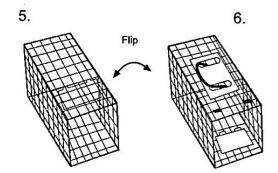
The cage should look like diagram 5. Its currently in an upside down position. Flip and turn the whole cage around so its the correct side up. You are now looking at the back of the cage.
