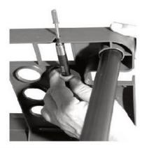
IMPORTANT:4. Use provided hardware to secure rack to wall or stable structure
