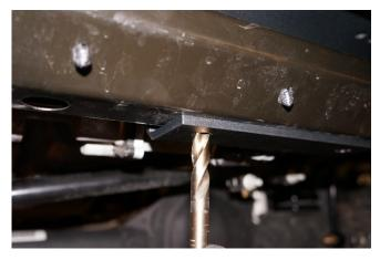
11. Locate to the 2 mounting points of the winch plate at the crash bar. Using the winch plate as a template, drill the 2 mounting points in the crash bar to 31/64". Clean and deburr the holes after drilling.
