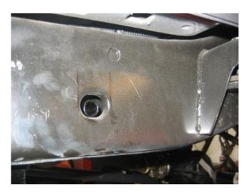
21. Refer to picture #7. Locate the outside frame crossmember gussets. These will be labeled driver and passenger side. Locate these two on their respective frame sides. Install the supplied 1/2" x 4-1/2" bolts with washers from the outside; they should go through the outside gusset, frame, spacer tube, and inside gusset respectively. Install the washers and start the nuts, but do not tighten at this time
