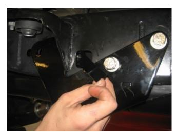
60. With the two-nut tab secure, place the one-nut tab through the square in the frame. Once start the supplied 9/16" bolt into the tab nut. Take precautions not to drop the tab nut into the frame.
