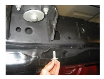
56. The passenger side lower long arm mount can be placed on the frame rail as shown in Picture #12. The straight line on the rear part of the bracket will sit flush against the front inside body mount. The gas tank mounting bolt should be threaded back into place. (Do not fully tighten). While threading the bolt back in place, push the bracket towards the frame to ensure correct placement. Just tighten slightly the bolt to insure the bracket is sitting flush to the frame rail
