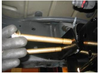
19. Refer to picture #4. This is the passenger side shown in the image below. Repeat the same process on the driver side. Do not fully tighten at this point, only start the nuts.
