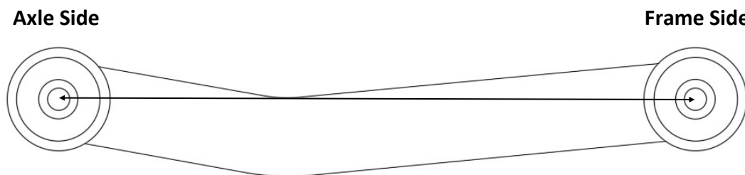
Lower Control Arm Measurement: 16-1/4" Center to Center Length
