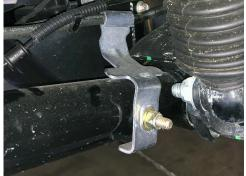
22. Install the supplied Rusty's Front Brake Line Extension Brackets where the front brake lines are attached to the frame with the use of the supplied hardware as well as the use of the factory hardware.
