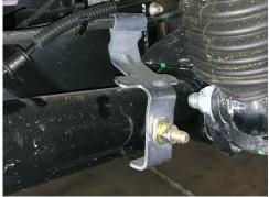
22. Install the supplied Rusty's Front Brake Line Extension Brackets where the front brake lines are attached to the frame with the use of the supplied hardware as well as the use of the factory hardware.
