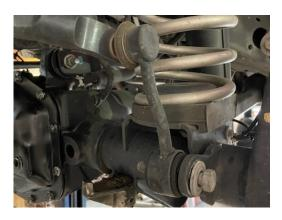
3. Locate the supplied driver's side relocation bracket (Note: It will have a larger inside slotted opening) and slide it over the factory sway bar axle tab location and install the supplied 1/2"-13 x 2" Length Grade 8 Hex Head Cap Screw, 1/2" SAE Flat Washer, and 1/2"-13 Grade 8 Hex Lock Nut as illustrated in the image below. Fully tighten hardware at this time.
