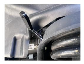
7. When disconnecting the sway bar links you can simply disconnect from the axle side and rotate the sway bar links up to the installed retention brackets and secure using the Retaining Clip removed from the axle side bullet pins.
