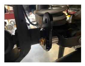
5. Install the supplied Quick Disconnect Bullet Pin and Lock Nut on both the passenger and driver side sway bar relocation brackets as shown in the image below. The bullet pins on each of the relocation brackets will point to the center of the vehicle. (**Note:** Make sure that the retaining clip hole is vertical when tightening the hardware.) Once tightened install the supplied Black Neoprene 3/4" ID x 1.37" OD Damping Washer on each pin.
