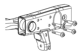
5. Install the supplied Rusty's JL Front Track Bar Frame Brace over the factory track bar mount and align the upper four mounting holes with the four steering box bolt hole locations and reinstall the factory hardware to secure the steering box and brace. Apply Blue Loctite to threads before reinstalling these bolts. (Note: Do not fully tighten the four bolts to the steering box at this time, only tighten enough to safely secure the steering box so that your assistant can let go.)
