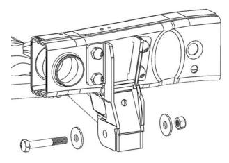
7. Install the supplied (Qty:1) 7/16"-14 x 1-1/4" Length Grade 8 Hex Head Cap Screw, (Qty:2) 7/16" SAE Flat Washer, and (Qty:1) 7/16"- 14 Grade 8 Hex Lock Nut to the hole location in the image below. (**Note:** Do not fully tighten hardware at this time.)
