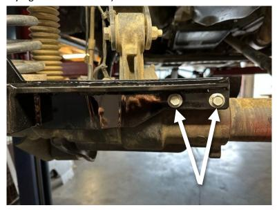
9. Install the supplied tube spacer in the factory track bar mounting location and install the supplied M14 x 2.00mm x 90mm Length Hex Head Cap Screw (Qty:1), Washers (Qty:2), Lock Nut. (Do not fully tighten at this time.)
