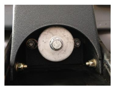
11. The holes now should be drilled 3/8" on each mounting point. Once all mounting points are drilled, debur the drilled holes for a smooth mounting surface.
