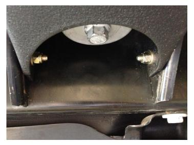
12. Install the 3/8" x 1-1/4" bolts, washer & nyloc nuts. Install at the 5 points and torque to 40 ft.-lbs.
