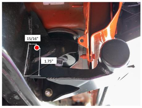
14. Drill the marked hole location to an 3/8" hole. We suggest drilling a pilot hole of 1/8" prior to drilling the hole to 3/8".
