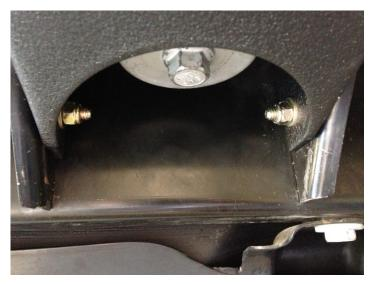
12. Install the 3/8" x 1-1/4" bolts, washer & nyloc nuts. Install at the 3 points and torque to 40 ft.-lbs.
